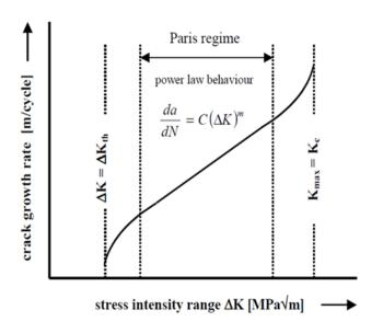
•FCG is due to the occurrence of several, interdependent, **damage mechanisms** at the crack tip zone.
