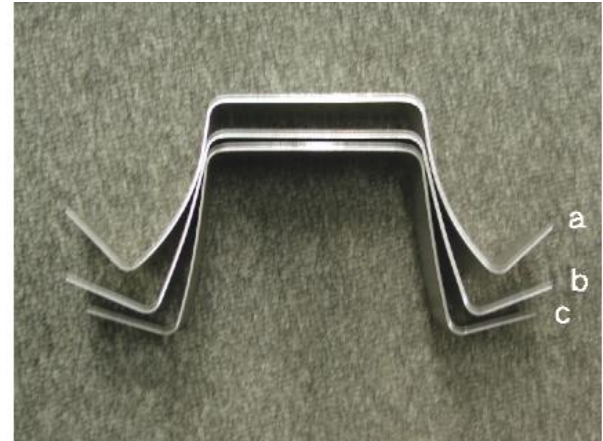
a: Aluminum alloy in cold forming b: Aluminum alloy in warm forming at 250°C c: Steel in cold forming
