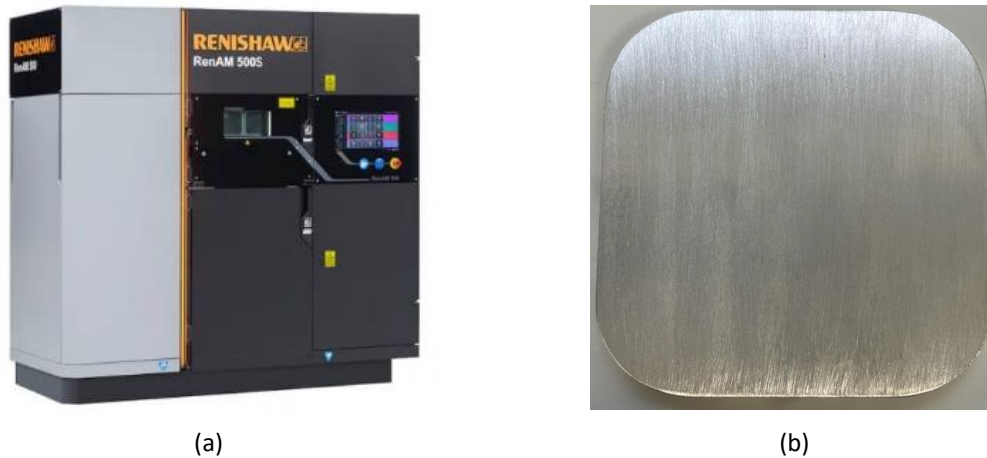
Figure 2.3. Renishaw system for L-PBF additive manufacturing: (a) RenAM 500S Flex; (b) substrate geometry used in the reduced build volume.
