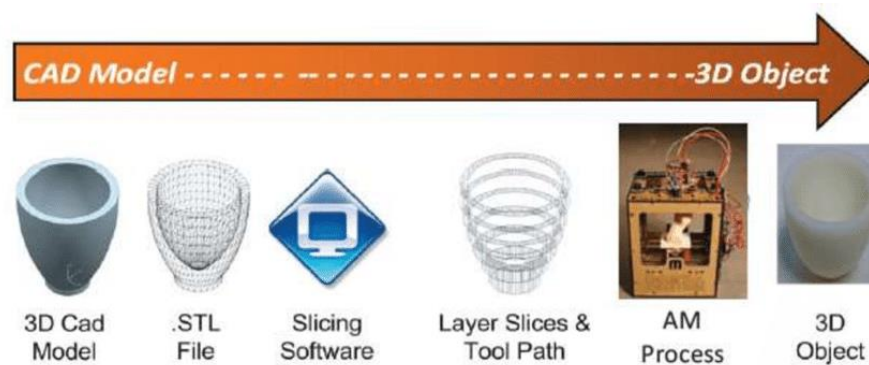
Figure 1.1. General process workflow of Additive Manufacturing from CAD model to 3D object [2].
