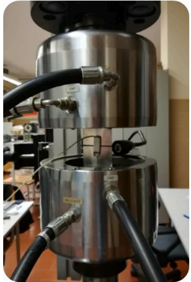
Fig. 4. Experimental set-up for FCG test using a MT specimen.
